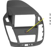
The built-in hazard button replaces the factory button that was integrated into the factory radio controls
