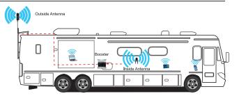
The Booster captures the signal from outside vehicle and boosts it to the phone. It takes the weak signal from your phone and boosts it back to the tower
